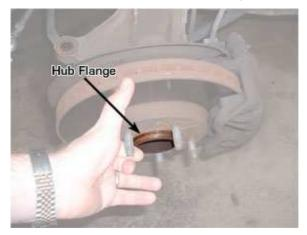
**Lug Centric** wheels are centered by the torque of the lug bolts; rather than the hub flange.
